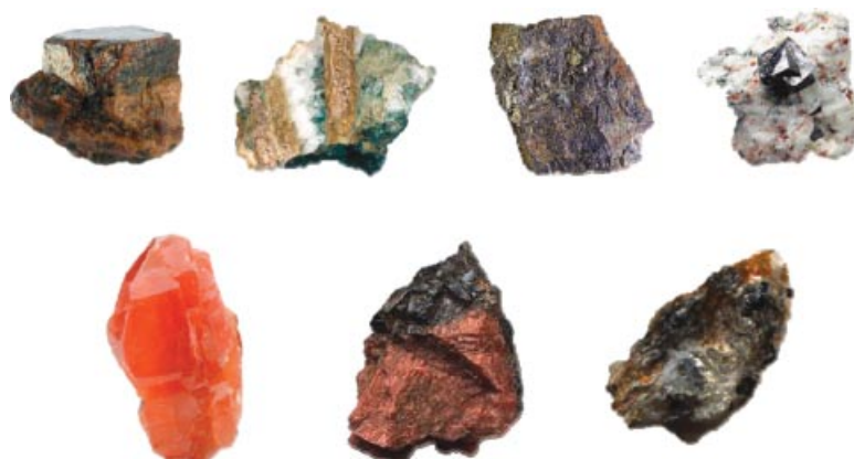
Fig. 2. Pictures of the currently exploited rare-earth minerals (from Wikipedia). Top row, cerium group, from left to right: bastnäsite, monazite, cerite, and loparite-Ce; bottom row, yttrium group, from left to right: xenotime, gadolinite, and euxenite.
